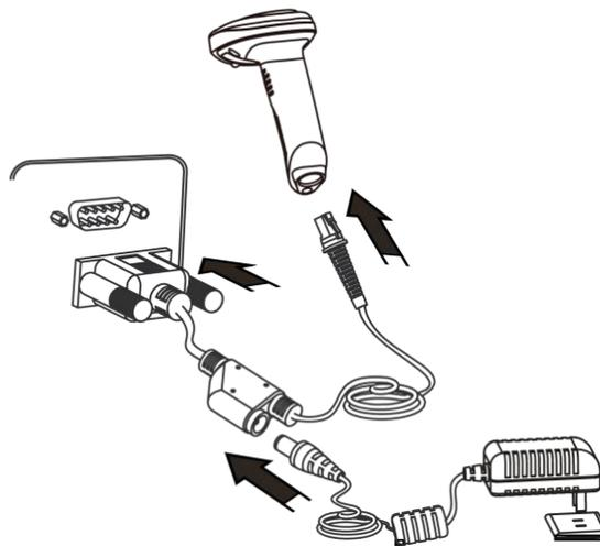
Connect the scanner to a Host through an RS-232 cable with RJ45, RS-232 and power connectors:
