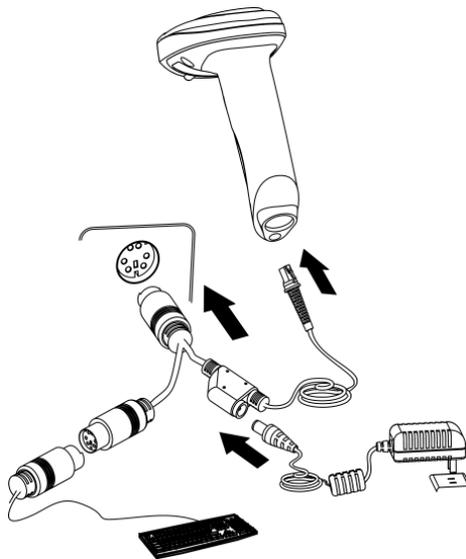
Connect the scanner to a Host through a PS/2 cable with RJ45 and PS/2 connectors and a power jack:
