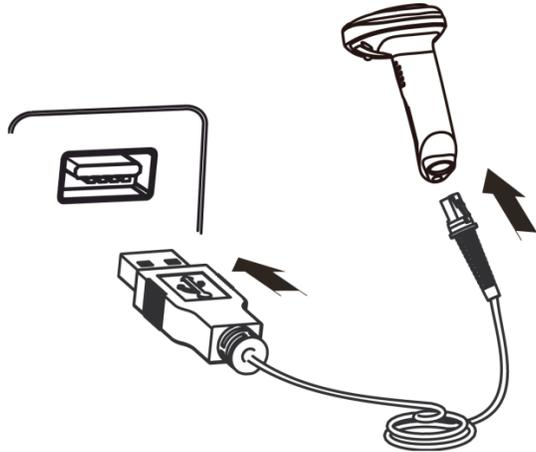
Connect the scanner to a Host through a USB cable with RJ45 and USB connectors:
